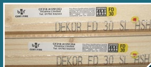
Photo 3. Important to make sure your fire-rated materials arrive on site with the right labels and certificates, are in good clean condition and with fire doors, that they are not fitted too early in the works, to avoid damage.
